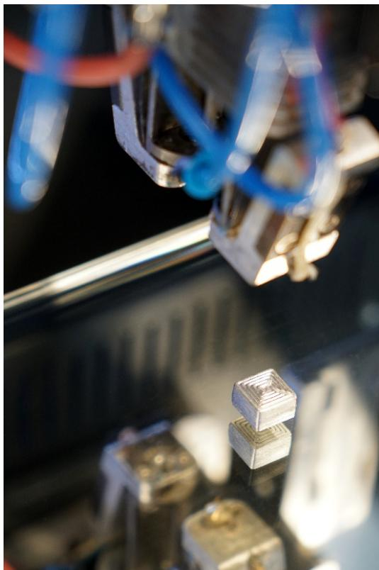
Hardmetal sample with complex geometry on FFF standard printer Hage3D 140 L, in which larger components can be perspective printed as well.
